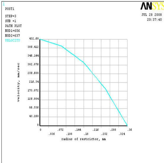
Fig. 16. Velocity profile of the fluid in the restrictor.
