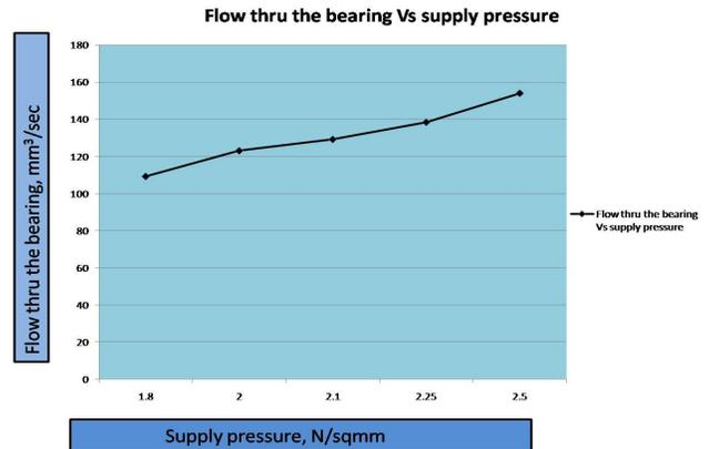
Fig. 18. Flow through the Bearing Vs Supply pressure.
