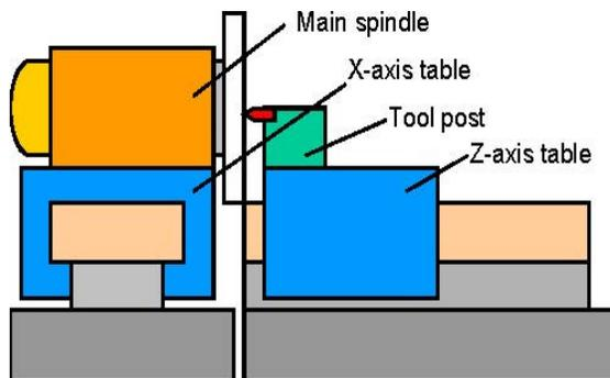
Fig. 2 Example of an ultra precision lathe.
