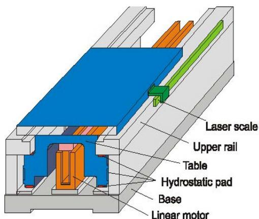
Fig. 3. The structure of the hydrostatic guide way was designed.
