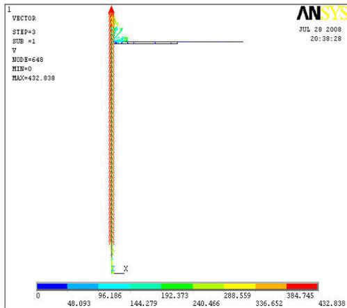
Fig. 17. Vector plot of velocity of the fluid in the restrictor.
