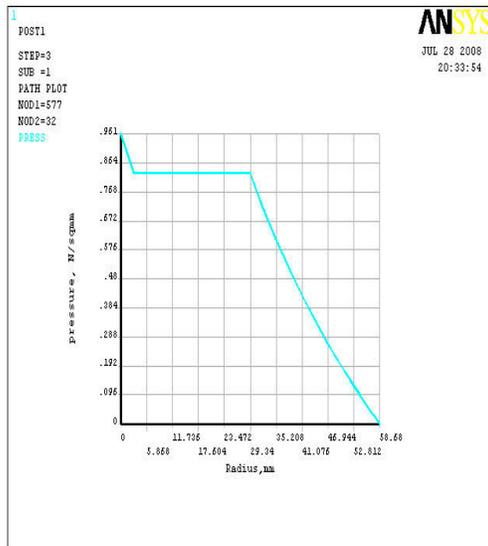
Fig. 15. Pressure acting on the slide Vs pocket radius.
