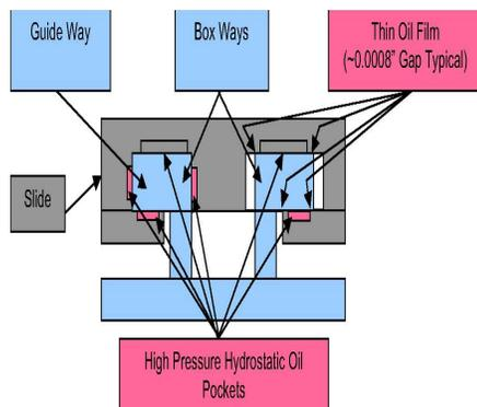
**Fig. 6.** The slide is supported and guided by these thin films of pressurized oil.
