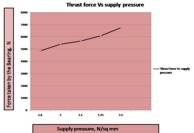
Fig. 19. Thrust force Vs Supply pressure.
