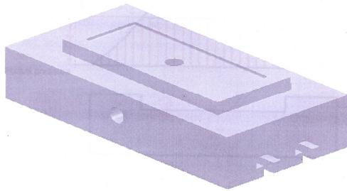
**Fig. 5.** A typical hydrostatic rectangular pad.
