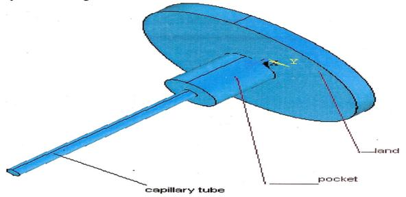
Fig. 10. 3-D Geometric model of the region.
