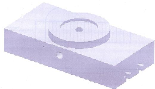
Fig. 4. A typical hydrostatic circular pad.
